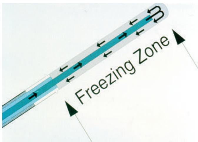
Figure 2b. Graphic demonstration of the circulation of the liquid nitrogen through the inner and outer cannula at the cryoprobe tip.
