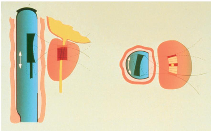
Figure 5. For BPH, the computer-controlled transducer ablates prostate tissue between the bladder neck and the verumontanum. Focal lesions are overlapped in linear rows (left) at each of the lateral sector positions (right) to create a volume lesion.
