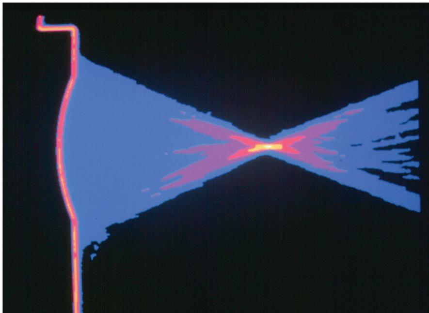
Figure 2. Color-coded Schlieren photograph demonstrates the discrete focusing ability of the HIFU transducer. Lethal zone is color-coded yellow and red. (Courtesy of Intec Research Company, Sunnyvale, Calif.)
