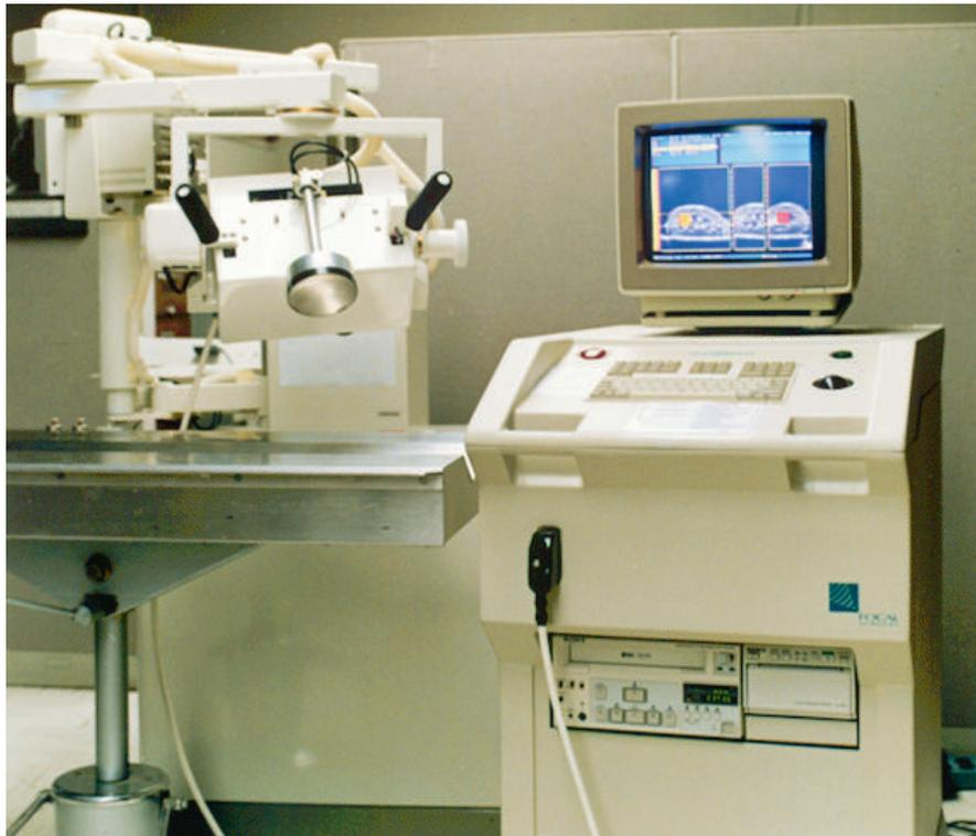
Figure 13. Prototype extracorporeal acoustic ablation device using a position-sensitive arm to accurately position the annular array imaging/therapy head. (Courtesy of the Indianapolis Center for Advanced Research, Indianapolis, Ind.)
