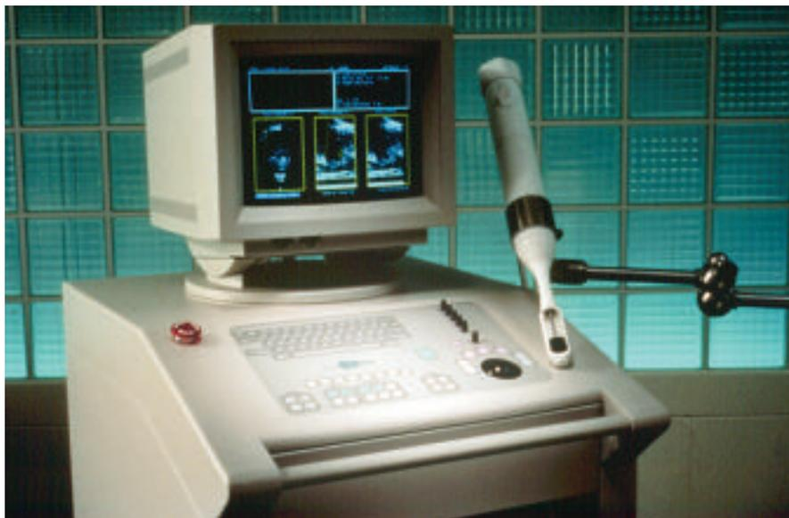
Figure 3. The Sonablate acoustic ablation system incorporates an endocavity probe that houses a dual function transducer that provides both imaging and HIFU for therapy.
