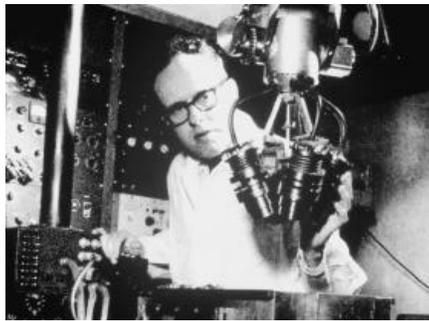
Figure 1. Professor William Fry pictured with an early HIFU device designed to focus the energy from four separate transducers into a single focal zone. (Courtesy of the Indianapolis Center For Advanced Research, Indianapolis, Ind.)
