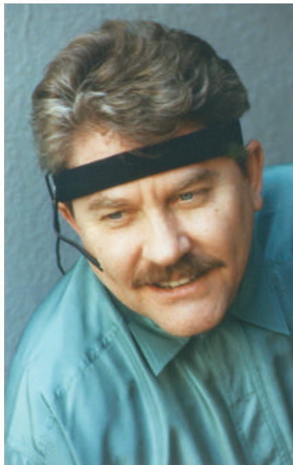
Figure 1. Headband with electrodes as an EOG controller. Another "drop-down" electrode, on the left side of the face, is necessary for three-dimensional eye controllers.
