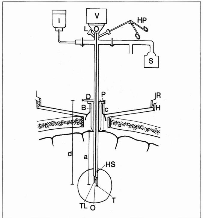
Figure 2d. Ultrasound stereotactic endoscopic microneurosurgery: H and R= fixation ring for ultrasound probe or neuro-endoscope. I= infusion system for the neuro-endoscope, L= Neodym YAG laser connector, O and V= connector for video system, S= suction system, D= tip of microbiopsy forceps, HP= microbiopsy forceps, TL= tip of microlaser tube.
