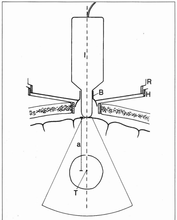
Figure 2b. Consecutive ultrasound stereotaxy: a= distance between brain surface and target point, B= ball joint, H= fixation ring for the ultrasound probe and biopsy instrument, 1= central ray of ultrasound probe, R= fixation ring, T= target point.
