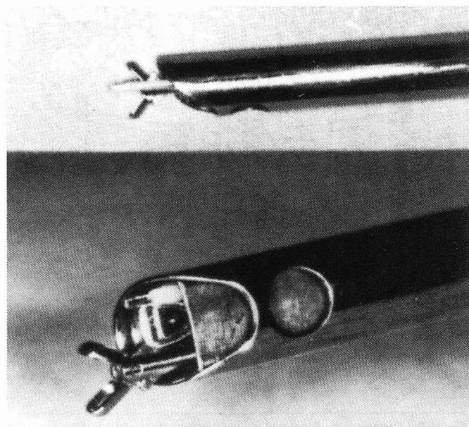
Figure 3d. Tip of endoscope with oblique end and additional suction channel, optic system, biopsy forceps and tip of laser probe.
