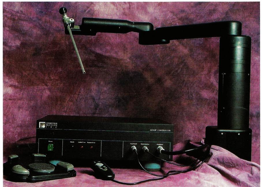
Figure 5. The AESOP computer controlled robot is shown here with the laparoscope support arm, computer control unit, foot and hand controls.
