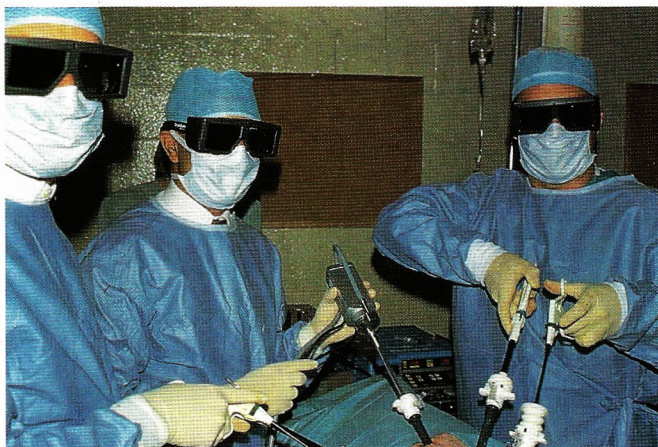
Figure 8. Shutter glasses being used with an "active" 3-dimensional display system.
