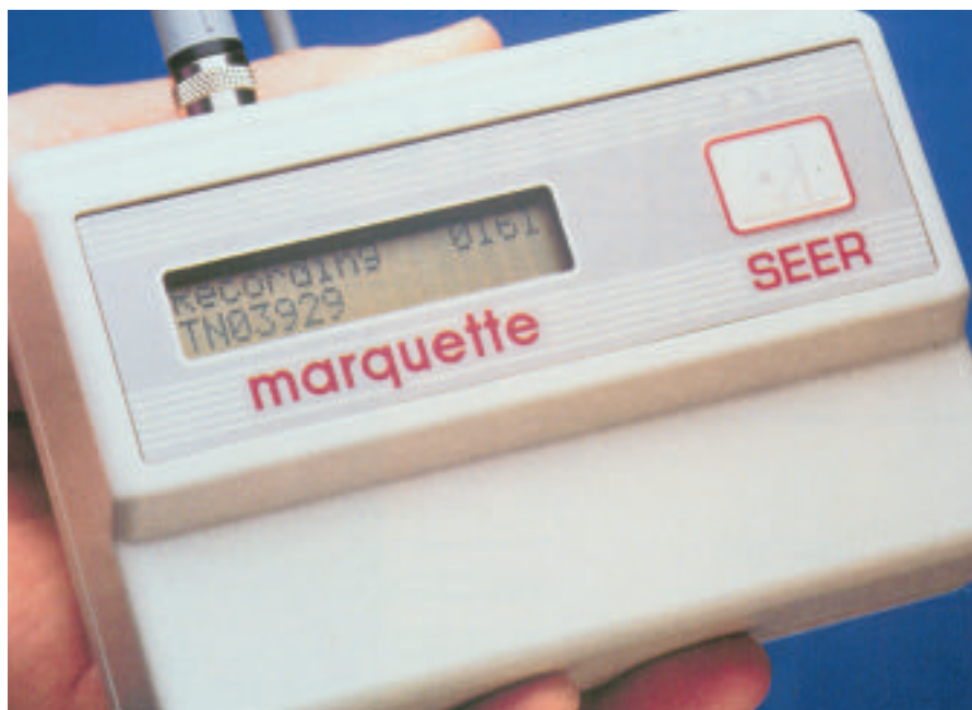
Figure 1. New digital technology allows sophisticated real-time ECG data analysis to be incorporated into portable Holter monitors. These devices have significant potential to be used for detecting postoperative episodes of silent myocardial ischemia which identify patients at highest risk for myocardial infarction.
